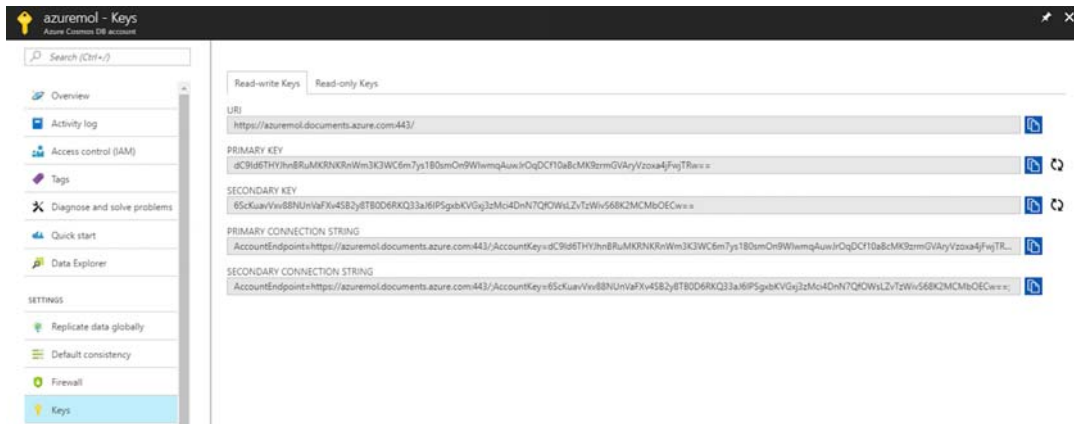
Figure 10.13 The Keys section of your Cosmos DB account lists the connection information and access keys. You need this information when you build and run applications, such as in the end-of-chapter lab.
